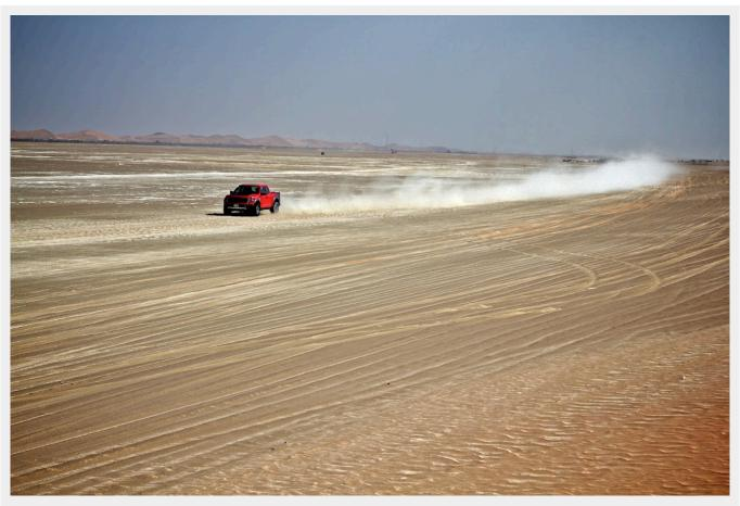
The suspension is simply amazing and high speeds off-road are possible. The secret of the Raptor's success lies in professional-grade racing suspension components: the front is coil-on-shock, long-spindle double-wishbone independent, aluminum lower control arm, forged-steel upper arm, FOX Racing Shox; and the rear is a Hotchkiss-type non-independent live, leaf springs and outboard shock absorbers, also running FOX Racing Shox.
