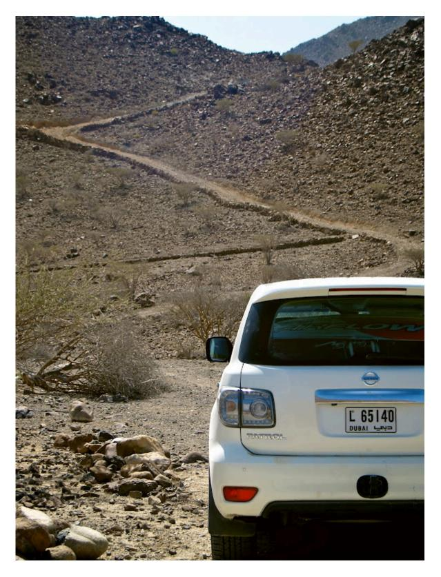
See that track cutting up the mountain in Wadi Al Helo? The Nissan Patrol crawled up with the sure-footdeness of a mountain goat, after plonking the central differential in low range, with traction control eliminating wheel slippage on the loose shale.
