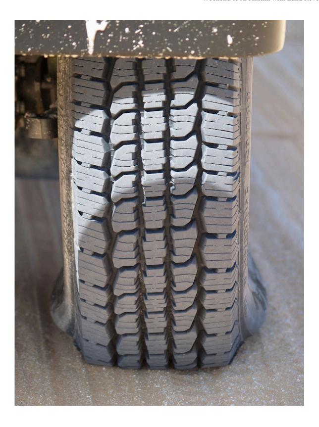
Deflating tyres is a good idea even if you feel the engine is powerful enough or the sand compact enough – the extra surface of rubber on the ground, called the footprint, will dramatically improve the flotation and the traction, which in turn means you can relax the engine and chug leisurely through the soft stuff instead of screaming along at high rpm all the time.
