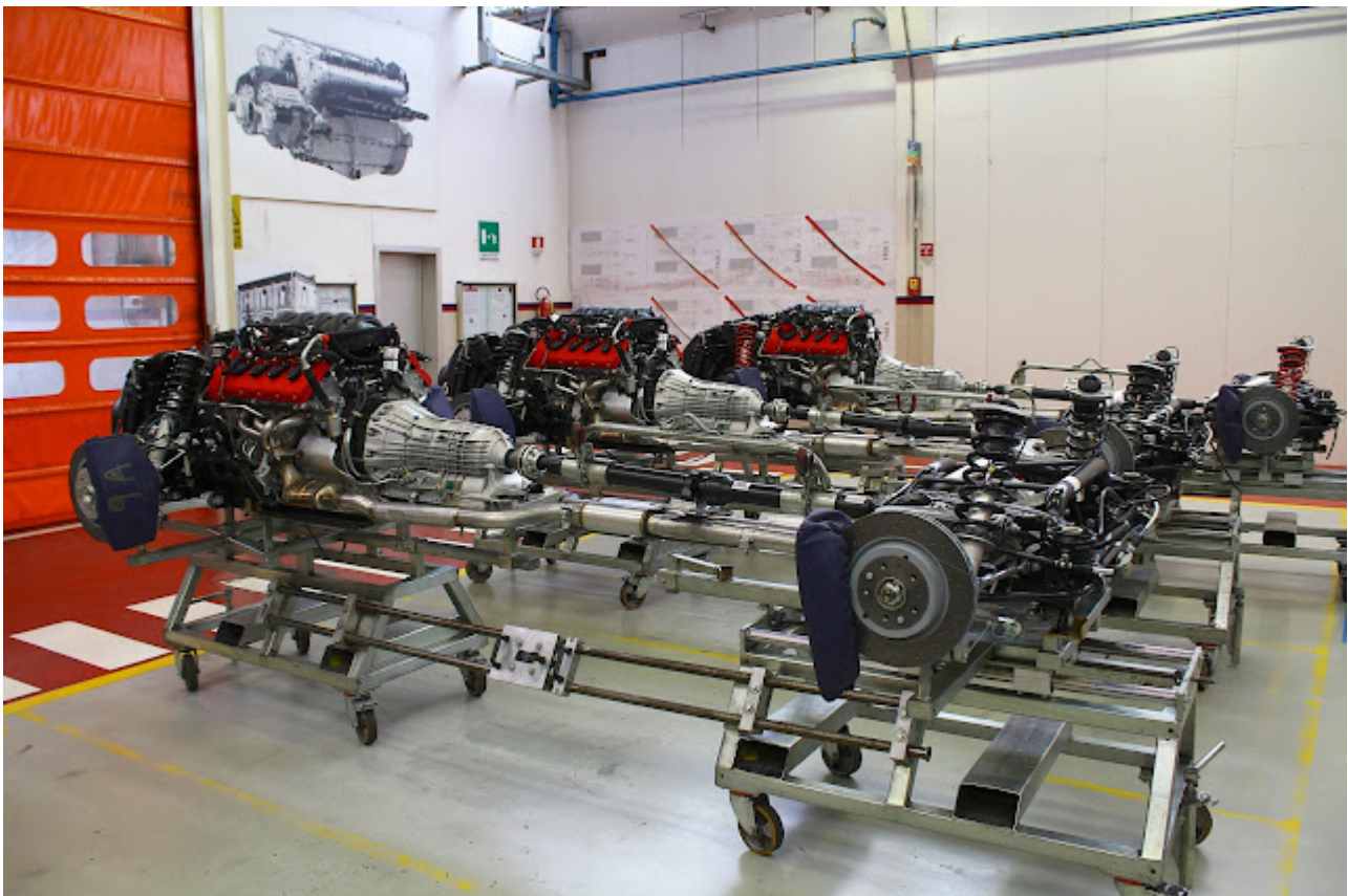
Transmission and engines come directly from Ferrari.
