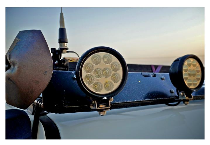
Up high on the roof rack they illuminate with a downwards perspective, useful to shine light into depressions in front of you, while down by the front grill the more powerful spot beams can aim for the horizon.
