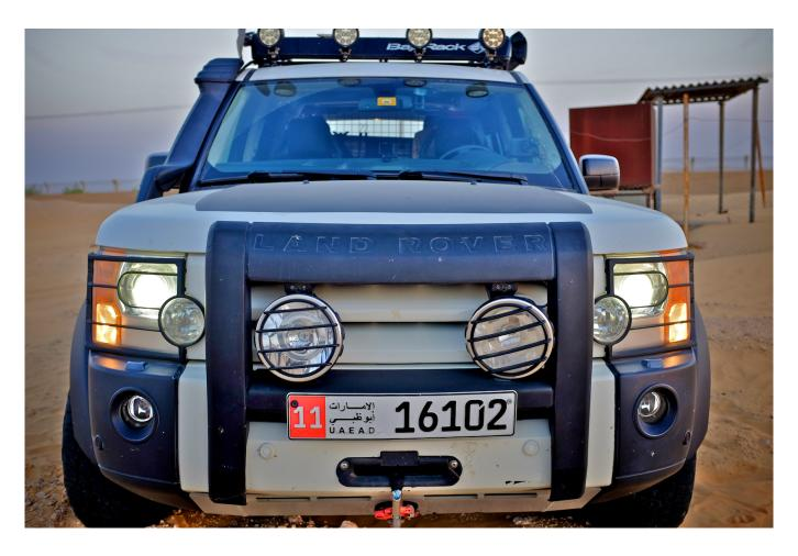
Stone guards give the needed protection, while a winch built into the bumper guarantees an exit from any sticky  $4 \times 4$  situation.
